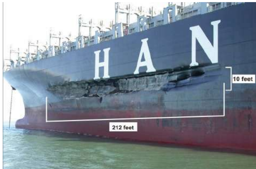
Damage to the forward port side of the Cosco Busan after the allision with the bridge tower.
